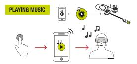
Once the Twiins® HF1.0 Dual + HF2.0 Dual is paired to a mobile phone capable or transmitting music through Bluetooth® A2DP, activate musi on the phone and it will immediately be heard through the Twiins® HF1.0 Dual + HF2.0 Dual device. Music and volume can only be controlled from the phone or device, depending on its features and configuration.
